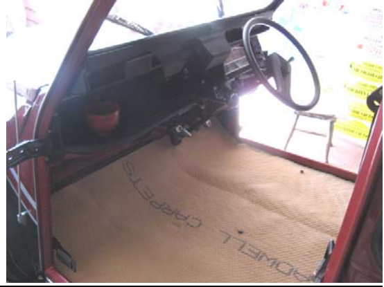
Floor pan re-painted ready for seats. Re-fit new underlay before mats refit.
