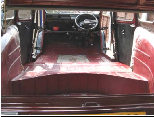
Floor pan re-painted ready for seats. Re-fit new underlay before mats refit.
