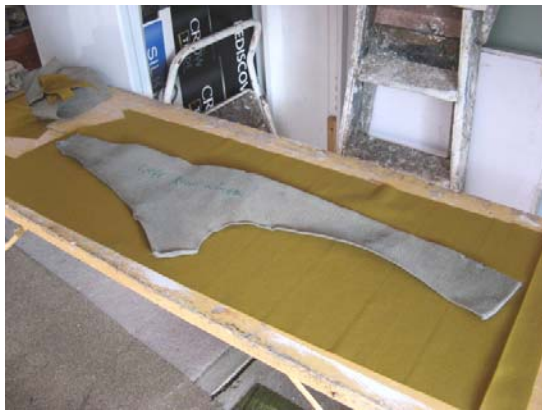
Cutting out new felt from old pattern. Refit new lining with the help of Spray Tac
