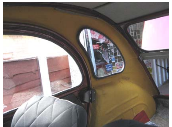
Cutting out new felt from old pattern. Refit new lining with the help of Spray Tac
